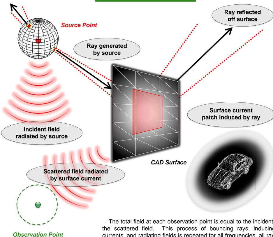
The total field at each observation point is equal to the incident field plus the scattered field. This process of bouncing rays, inducing surface currents, and radiating fields is repeated for all frequencies, all rays, and all observation points.
