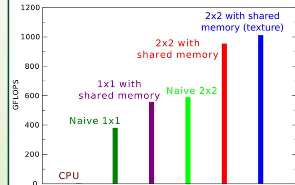
Performance using a GeForce GTX 480 with  $N=1024$  ( $n_s=512$ ) and  $F=12$ . The 1x1 or 2x2 labels the register tile size. The naïve case represents all threads loading all data, the shared memory uses the shared memory for an extra level of tiling.
