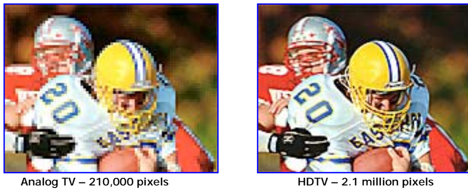
Figure 4. Pixels in Analog TV vs. HDTV
