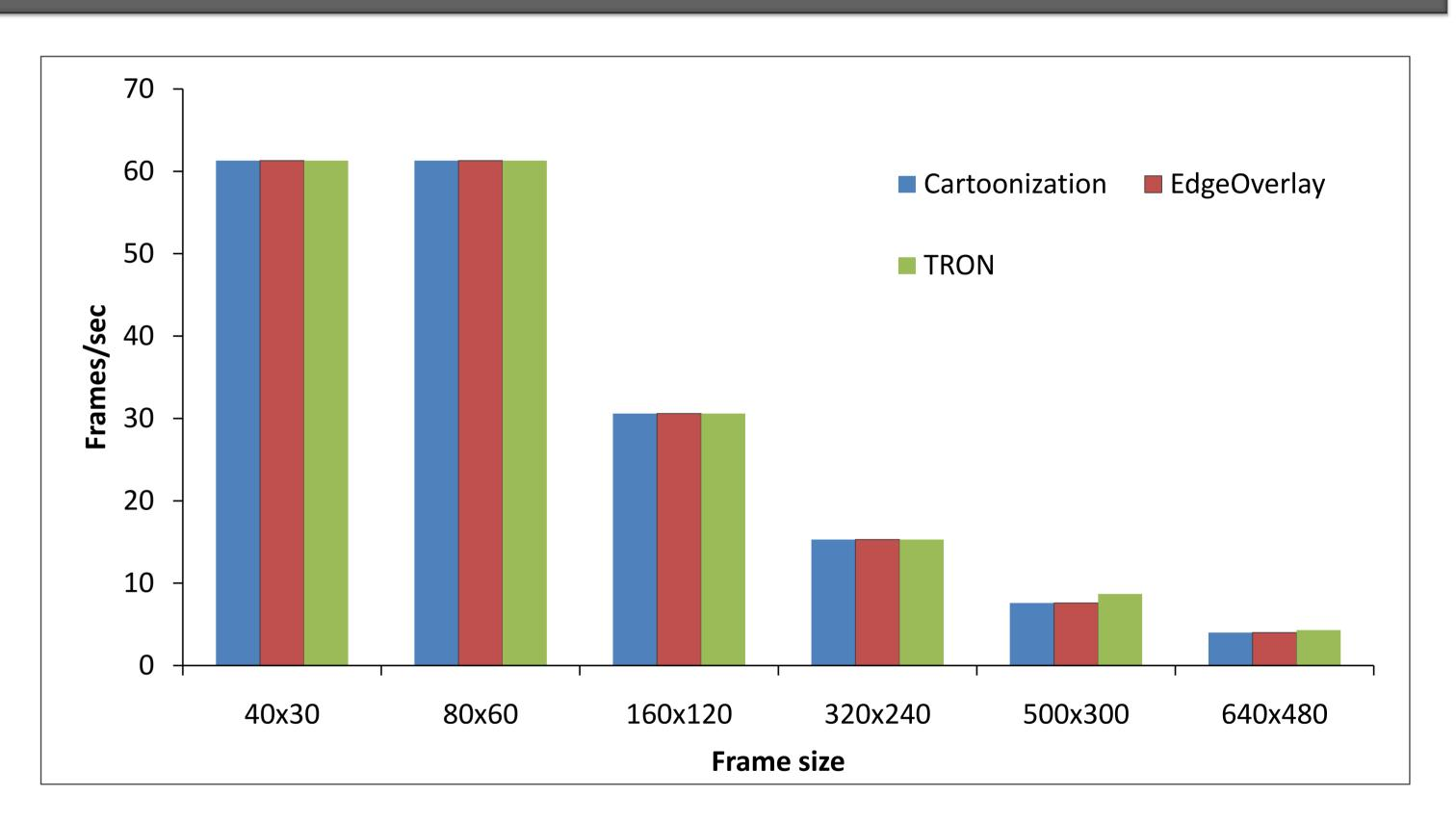
For the two smaller images the frame rate is around 61 fps which is the maximum value that the GPU can reach. For bigger image sizes the frame rate rapidly becomes really low (around 7fps for 500x300 and around 4fps for 640x480). However, with the release of the Tegra II, we can expect to obtain results much closer to real time.
