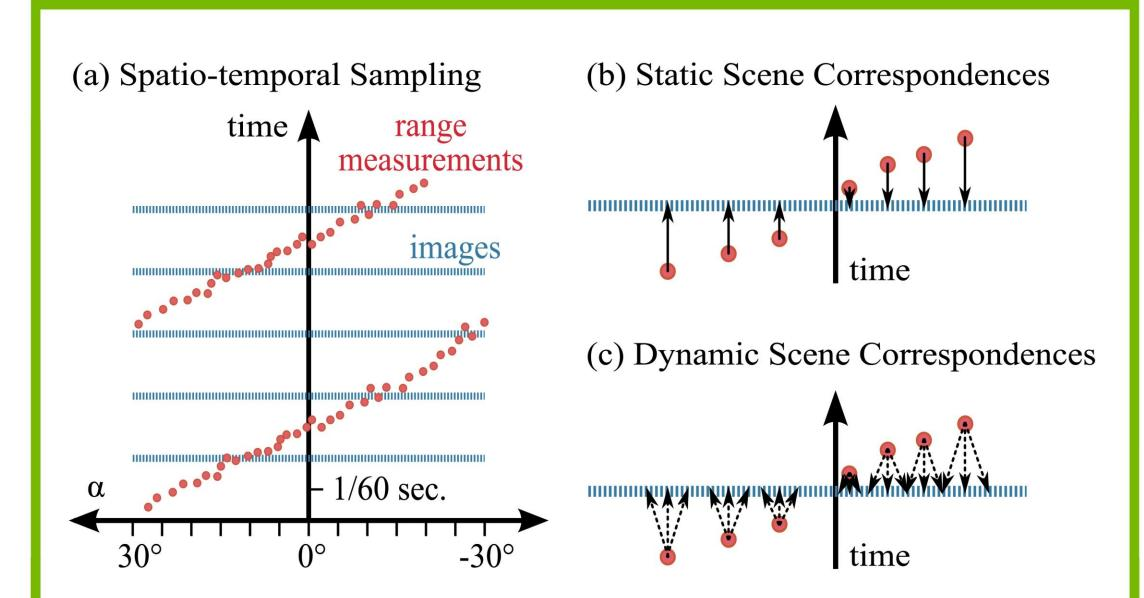
The fusion of image and range information is difficult because different parts of the scene are observed at different points in time. (a) visualizes the spatio-temporal sampling behavior of cameras and typical range scanning devices. (b) shows that correspondences between measurements are easy to establish for static scenes and (c) shows that this is not the case for dynamic scenes, since a measured object may have moved in space.
