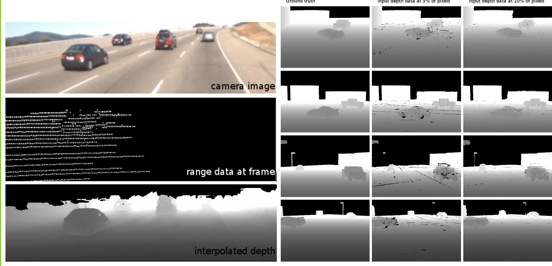
For any given camera frame, we can recover an accurate, dense depth map. The depth map shown in the lower left panel corresponds to a single camera frame from a sequence of highway images, recorded from a mobile platform. The right images are depth maps generated from synthetic data of increasing density. We can generate a depth map for an arbitrary camera frame even if the coincident depth data is sparse, or missing, using depth data from neighboring frames.
