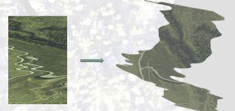
The images above show an example of applying georeferencing in rectifying a line scanned image severely disturbed by aircraft movement. Interpolation along the line is performed "automatically" in the texture mapping, which is "instantaneous"
