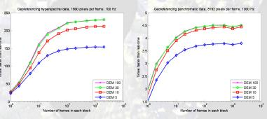
The figures above show that we for full resolution frames are able georeference faster than real-time. Optimal performance is reached for around 1 s large blocks, with a processing rate of about 35 Mpixel/s on a DEM corresponding to DTED level 2.
