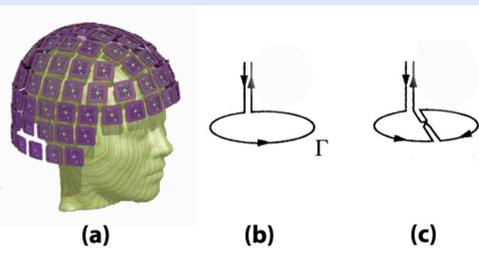
(a) 306 MEG sensors (b) Magnetometer (c) Planar Gradiometer
