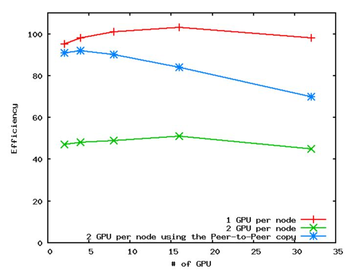
Efficiency with up to 32 (2070) GPU for a  $512^3$  system.
