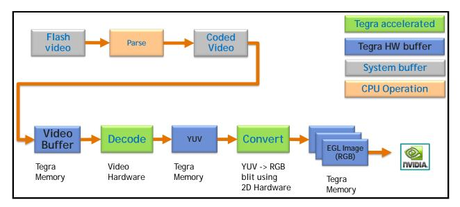
Figure 10 Flash Video Acceleration on NVIDIA GeForce GPU core
