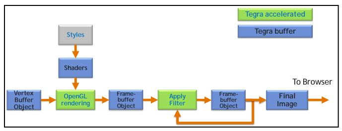
Figure 9 Acceleration of Flash graphics on Tegra GeForce GPU
