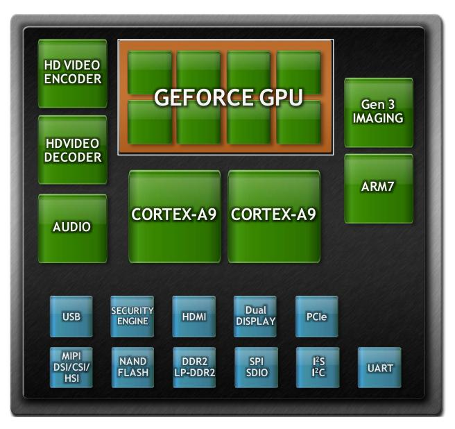
Figure 1 NVIDIA Tegra 2 with GeForce GPU
