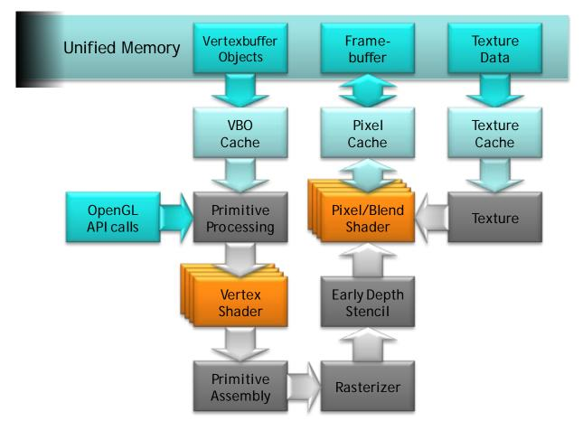
Figure 4 GeForce GPU Architecture in NVIDIA Tegra
