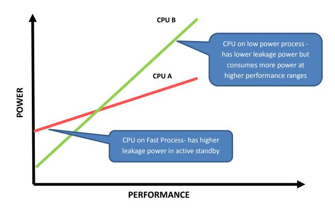
Figure 2 Mobile CPU Power-Performance curves
