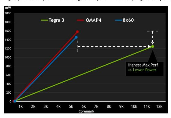
Figure 8 Tegra 3 power consumption delivering maximum quad core performance<sup>8</sup>
