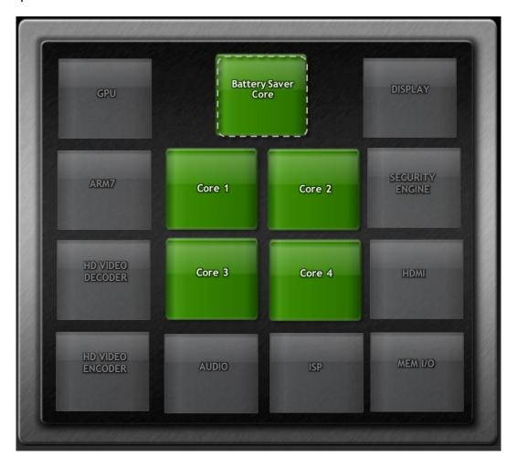
Figure 3 Low Power Battery Saver CPU on Tegra 3
