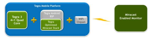
Figure 2 Tegra Miracast Wireless Display Topology
