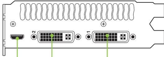
**DVI connector** for digital displays. Using the DVI-to-HDMI adapter, you can connect to HDTV. Using a DVI-to-VGA adapter, you can connect a second VGA display.
