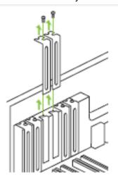
Remove two adjacent slot covers that corresponds to the PCI-Express slot you are installing the TITAN Xp graphics card in.
