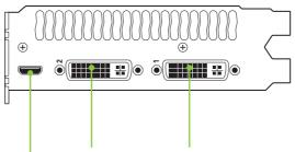
**DVI connector** for digital displays. Using the DVI-to-HDMI adapter, you can connect to HDTV. Using a DVI-to-VGA adapter, you can conected a second VGA display.
