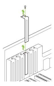
5 Plug the graphics card into the Primary PCI Express x16 slot on your motherboard. This is often the slot closest to the CPU but may be the second or third slot. Look for the slot labeled ×16. It will likely be the only PCI Express slot with a retention lever on the end of the slot (or the one closest to the CPU.
