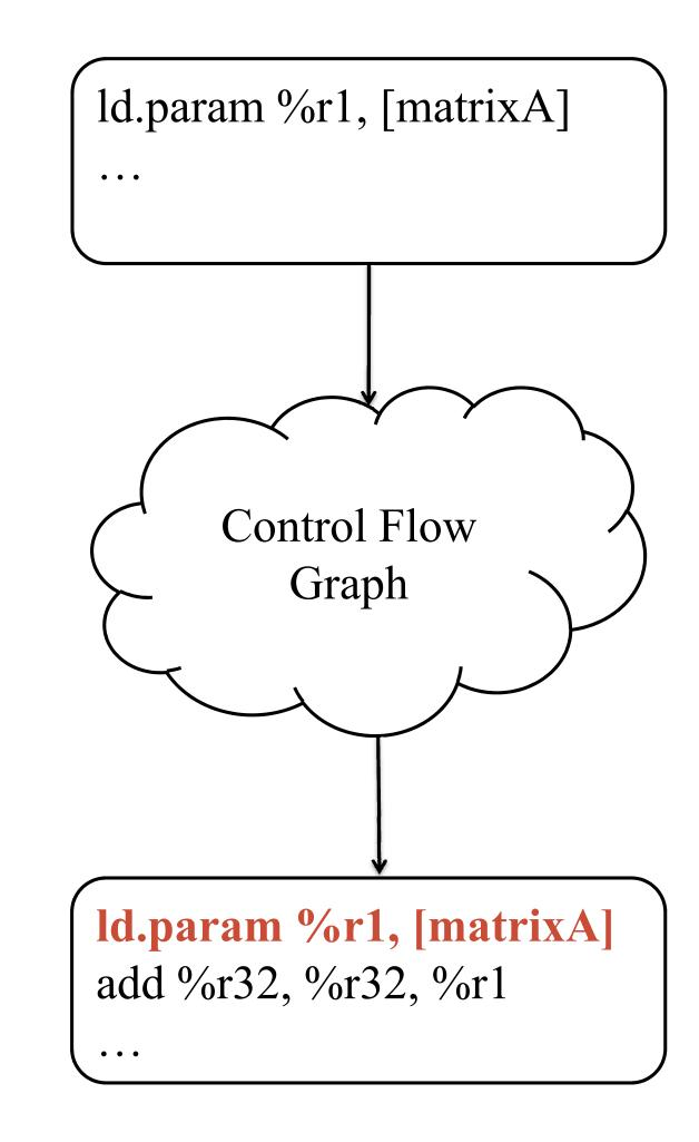
We rematerialize memory operations for loading parameters and special registers (e.g. threadId, blockId).
