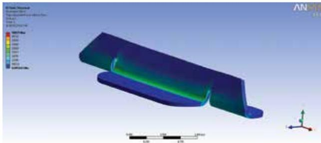
Sample analysis image of a component of the wheels for the new rover
