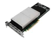
that includes the Dynamic Parallelism and Hyper-Q features. With more than one teraflop peak double precision performance, the Tesla K20 is ideal for a wide range of high performance computing workloads including climate and weather modeling, CFD, CAE, computational physics, biochemistry simulations, and computational finance.
