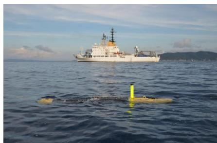
*High-resolution, high-frequency synthetic aperture sonar (SAS) with GPU acceleration on the MUSCLE autonomous underwater vehicle is making the seas safer for travel.*
