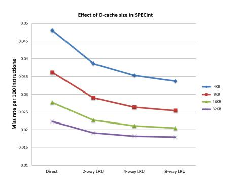
Figure 6 Impact of Data Cache size on cache miss rates and CPU performance
