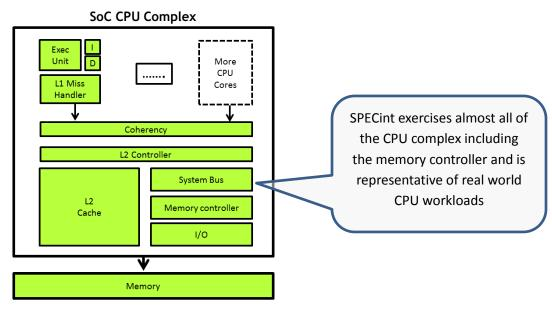
Figure 3 SPECint exercises the entire CPU complex and has workloads that are similar to real world applications
