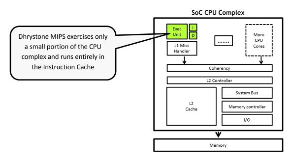
Figure 2 Dhrystone MIPS benchmarks only a small section of the CPU complex
