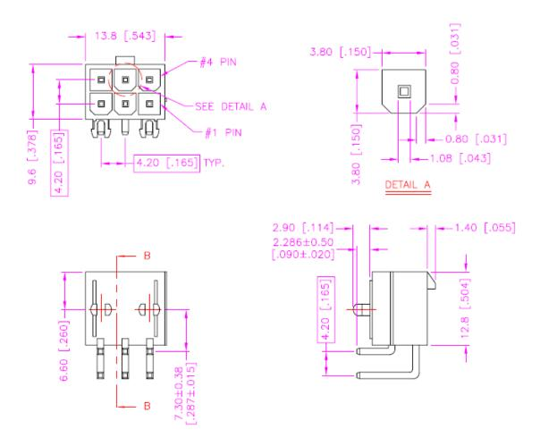
Figure 4. 6-Pin PCI Express Power Connector
