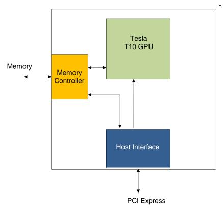
Figure 1. Tesla C1060 Block Diagram
