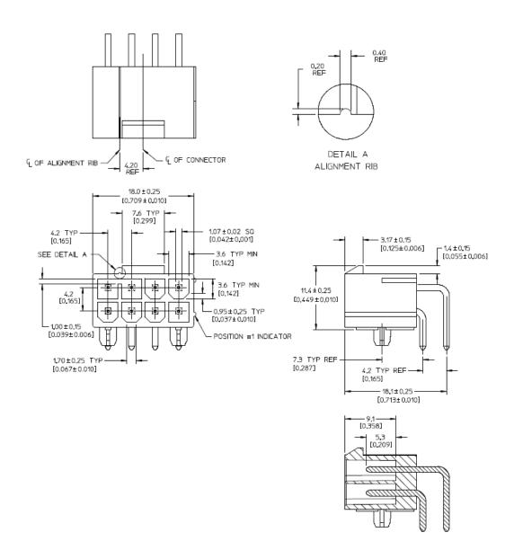
Figure 5. 8-Pin PCI Express Power Connector
