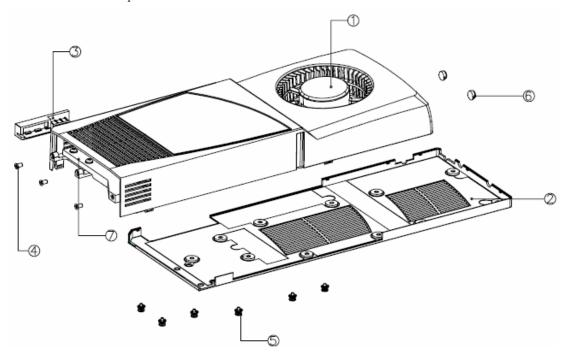
Figure 7. TM72 Active Fan Sink
