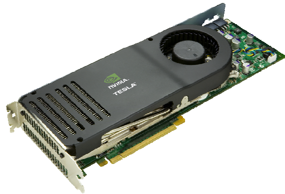
Figure 2-3: Tesla C870 GPU
