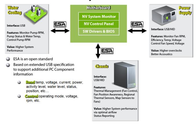
Initially ESA components will be comprised of chassis, power supplies, and water cooling components. Thanks to ESA's unique and flexible architecture, these components will be able to provide a wide array of information to the user. Here, data ranging from temperatures, fan speeds, and voltages will be relayed real-time to the user giving them the most current system status possible. Specifically, the reported data points for the appropriate hardware are listed below:
