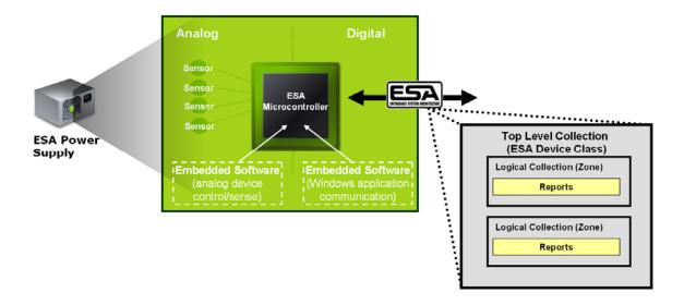
The ESA architecture is designed to facilitate a well-defined protocol for communicating information about sensors and controls within an ESA device. This communication is enabled by embedding a microcontroller into the enabled components. The microcontroller integrates a USB 2.0-compliant full speed device controller which is used as the primary communication channel between the PC
