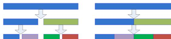
Left: Traditional divide and conquer methods split up data into separate arrays and recursively run an algorithm on the sub-arrays until the problem is solved. While this makes sense on CPUs, it is very hard to map efficiently onto GPUs.
