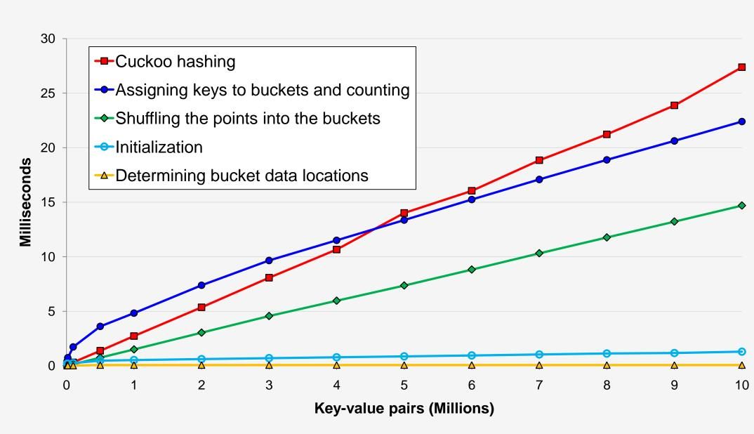
Timing for each stage of our algorithm for increasingly large input of random keys. We see roughly linear scaling for each stage.
