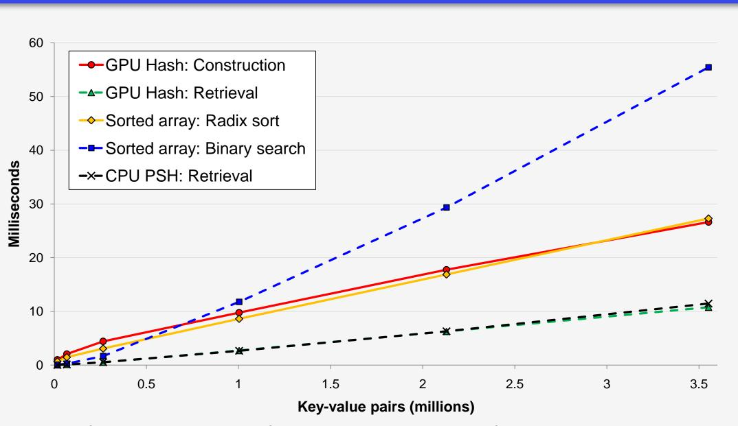
Timings for increasingly finer voxelizations of Lucy. We compare against a sorted list, using binary searches for retrieval. Construction takes roughly the same amount of time as the radix sort, while our retrievals are consistently faster than binary searches for random access.
