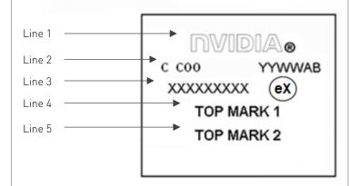
Pin 1: Location of Pin 1 in upper left when reading the
