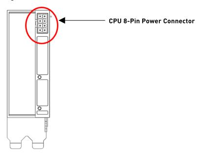
Table 7 lists supported auxiliary power connections for the NVIDIA A100 80GB GPU card.
