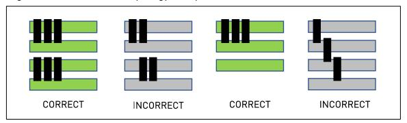
For systems that feature multiple CPUs, both A100 80GB cards of a bridged card pair should be within the same CPU domain—that is, under the same CPU's topology. Ensuring this benefits workload application performance. There are exceptions, for example in a system with dual CPUs wherein each CPU has a single A100 80GB PCIe card under it; in that case, the two A100 80GB PCIe cards in the system may be bridged together.
