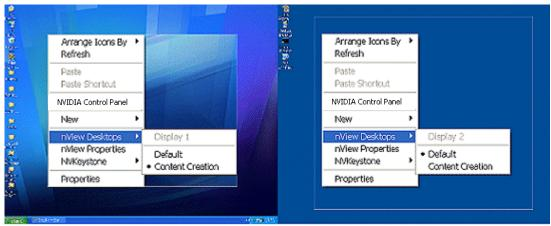
Figure 6.9 Opening Separate Desktops on Separate Display Screens
