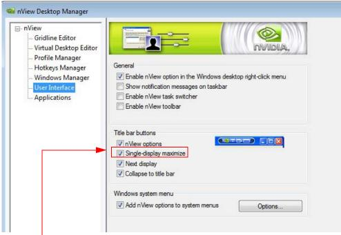
"Single-display maximize" check box is available only under nView Span modes.
