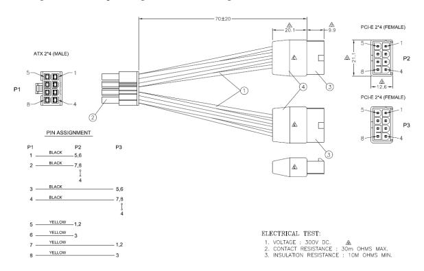
Figure 9. CPU 8-Pin to PCIe 8-Pin Dongle
