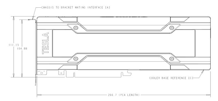
Figure 6. Tesla M60 Board Dimensions (With Optional I/O Bracket)
