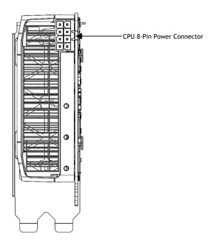
Figure 8. CPU 8-Pin Power Connector
