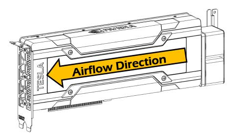
Figure 4. Tesla M60 (PG402 SKU 80): Right-to-Left Active Airflow with Straight Extender
