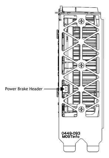
Figure 7. Power Brake Header
