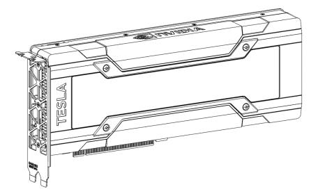
Figure 1. Tesla M60 Board (With Optional I/O Bracket)
