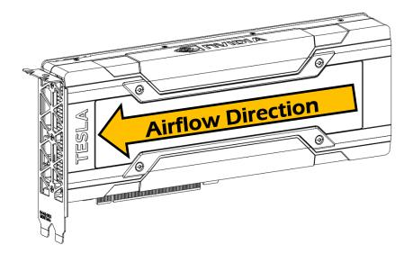
Figure 3. Tesla M60 (PG402 SKU 60): Right-to-Left Airflow
