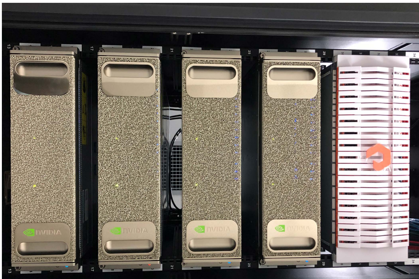
AIRI Solution with 4 NVIDIA DGX-1 and Pure Storage FlashBlade
