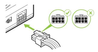
GeForce RTX 2060 SUPER graphics card requires one 8-pin PCI Express power plug from the system power supply.
