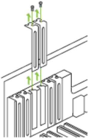
Remove two adjacent slot covers that corresponds to the PCI-Express slot you are installing the GeForce GTX graphics card in.
