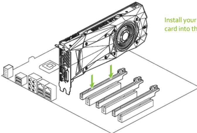
Install your first GeForce GTX 1080 graphics card into the Primary PCI Express x16 slot.
