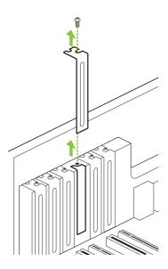
Plug the graphics card into the Primary PCI Express x16 slot on your motherboard. This is often the slot closest to the CPU but may be the second or third slot. Look for the slot labeled x16. It will likely be the only PCI Express slot with a retention lever on the end of the slot or the one closest to the CPU.
