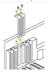
Remove two adjacent slot covers that corresponds to the PCI-Express slot you are installing the TITAN X graphics card in.
