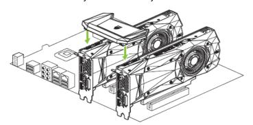
2-way SLI configuration: Install your second TITAN X graphics card into the outer PCI Express x16 slot (the outer slot is the one farthest away from the CPU).
