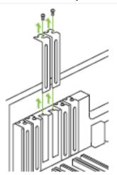
Remove two adjacent slot covers that corresponds to the PCI-Express slot you are installing the TITAN Xp graphics card in.
