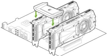
2-way SLI configuration: Install your second TITAN Xp graphics card into the outer PCI Express x16 slot (the outer slot is the one farthest away from the CPU).
