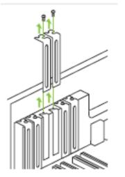
Remove two adjacent slot covers that corresponds to the PCI-Express slot you are installing the GeForce GTX graphics card in.
