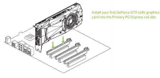
**Note:** It is recommended that you install the graphics card into the primary PCI Express x16 slot. If you install the graphics card into the secondary slot, your system may not recognize the graphics card and there will be nothing displayed on the monitor.
