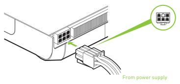
If your power supply needs an additional 6-pin power connector, you can use the included 4-to-6 pin adapter. Make sure to connect each 4-pin connector to a separate PSU cable.
