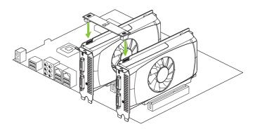
7 Connect one 6-pin PCI Express auxiliary power connectors coming from the computer power supply to the connectors on the top edge of on the top edge of the GeForce GTX 550 Ti graphics card.
