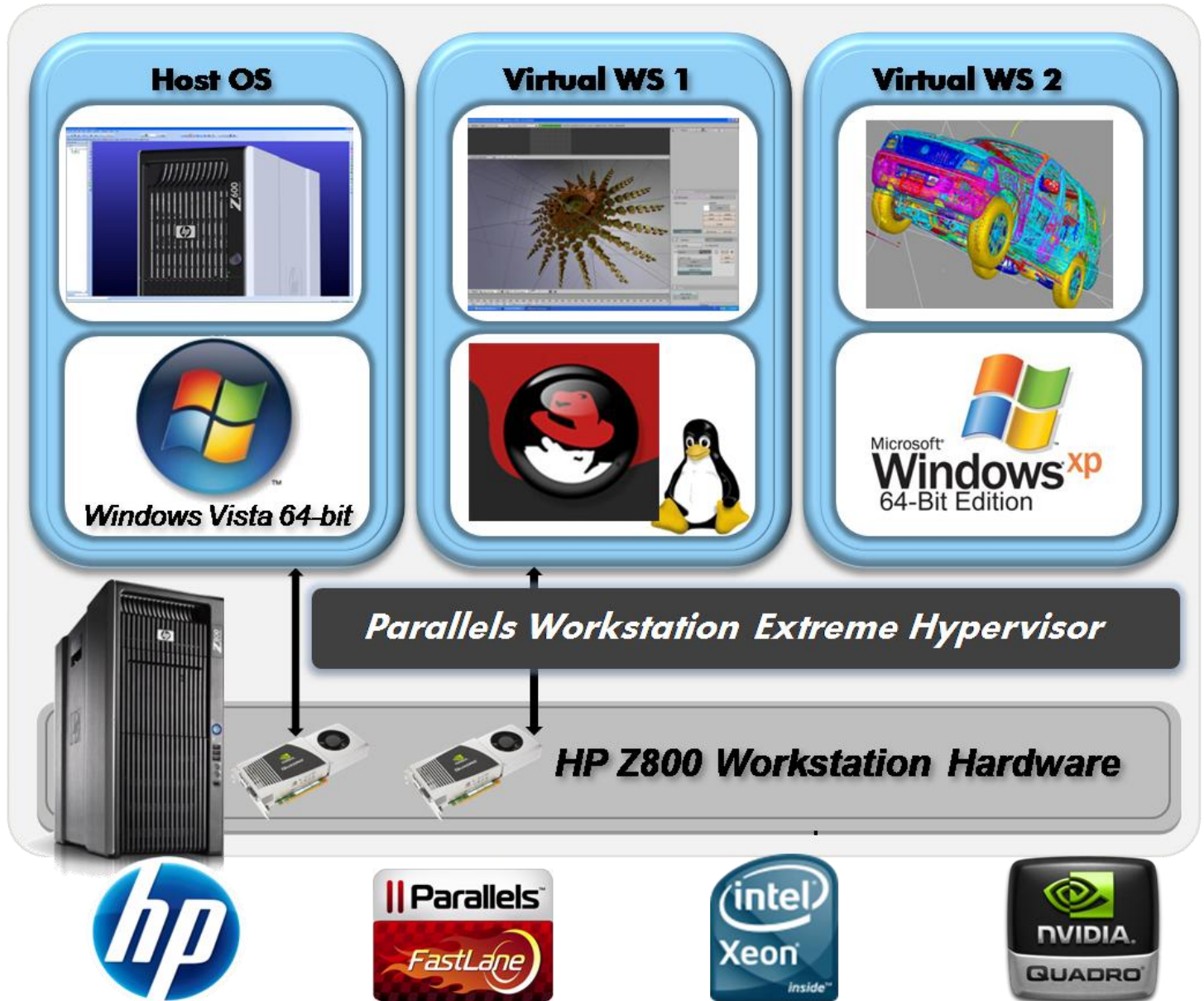
Figure 1: Block Diagram. One graphics card is used by the Host OS. A second graphics card is mapped to a virtual workstation
