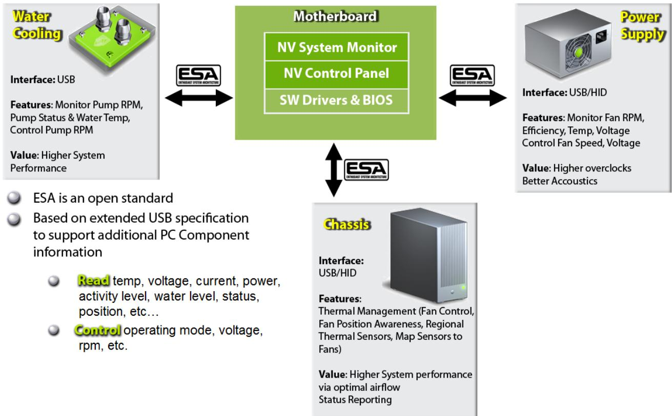
Initially ESA components will be comprised of chassis, power supplies, and water cooling components. Thanks to ESA's unique and flexible architecture, these components will be able to provide a wide array of information to the user. Here, data ranging from temperatures, fan speeds, and voltages will be relayed real-time to the user giving them the most current system status possible. Specifically, the reported data points for the appropriate hardware are listed below:
