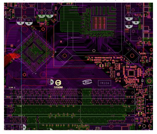
Figure 1 – NVIDIA nForce 790i Ultra SLI Motherboard Layout (DDR3 Memory Interface)
